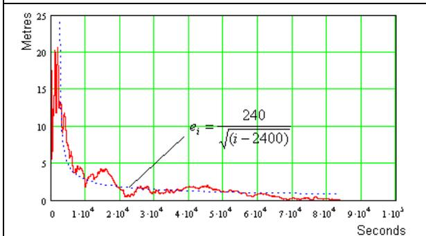
**Fig. 5: GPS with SA - the effect of position averaging, linear scales**
