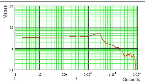
**Fig. 4: GPS without SA - the effect of position averaging, logarithmic scales**
