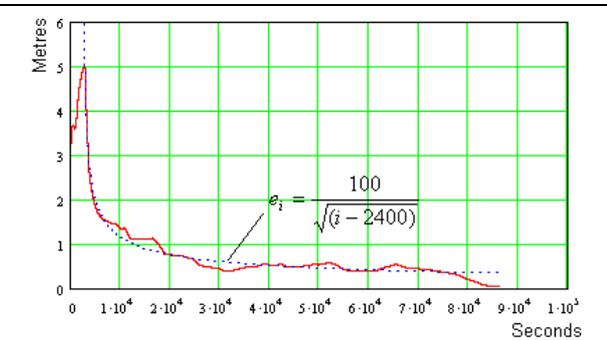
**Fig. 6: GPS without SA - the effect of position averaging, linear scales**
