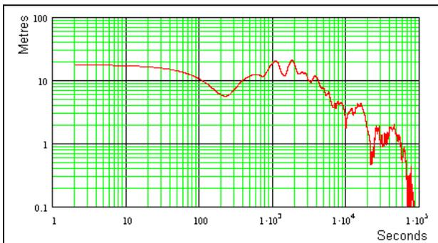
**Fig. 3: GPS with SA - the effect of position averaging, logarithmic scales**
